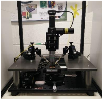
Probe station to measure both the electrical and optical characteristics of flexible and wearable optoelectronic devices (photo courtesy of Nathan Youngblood)
