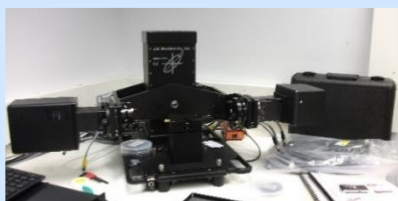
Woollam RC2 spectroscopic ellipsometer to measure advanced samples and nanostructures
