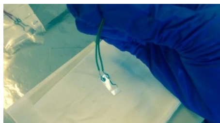
Figure 10 A PEDOT interdigitated electrode device connected to wires and ready for test
