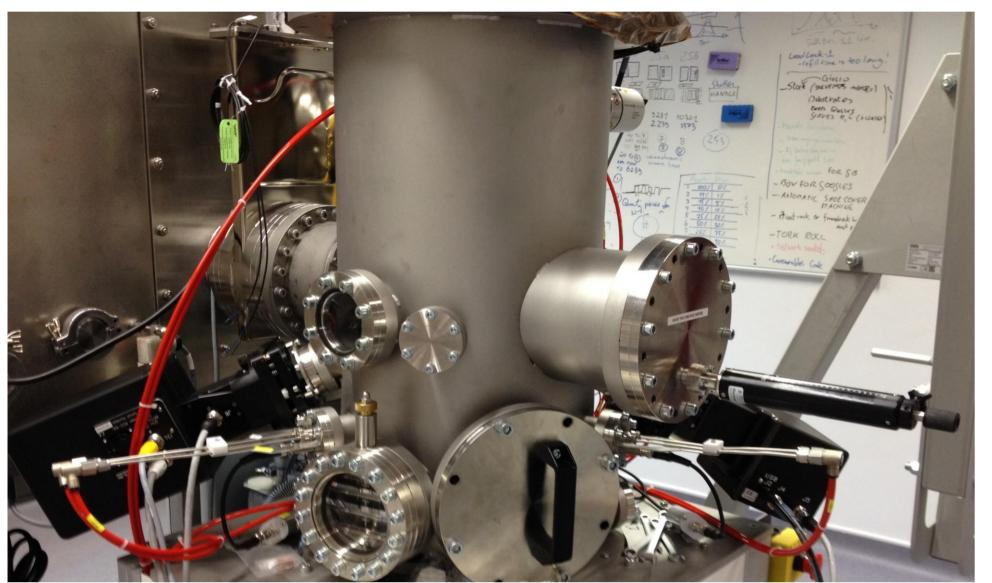
Vacuum chamber with mounted ellipsometer for *in situ* monitoring
