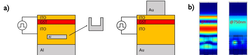
**Figure 2.** a) (left) Introduction of an embedded split ring resonator (SRR) array into the display structure and (right) alternative metamaterial array structure consisting of patterned metal strips on top of the upper ITO layer. Metal used in the structure on the left is aluminium whereas on the right is gold. b) Electric field plot at the excitation wavelengths for maximum (750nm) and minimum (475nm) interaction of the resonance of the cavity with the SRR.
