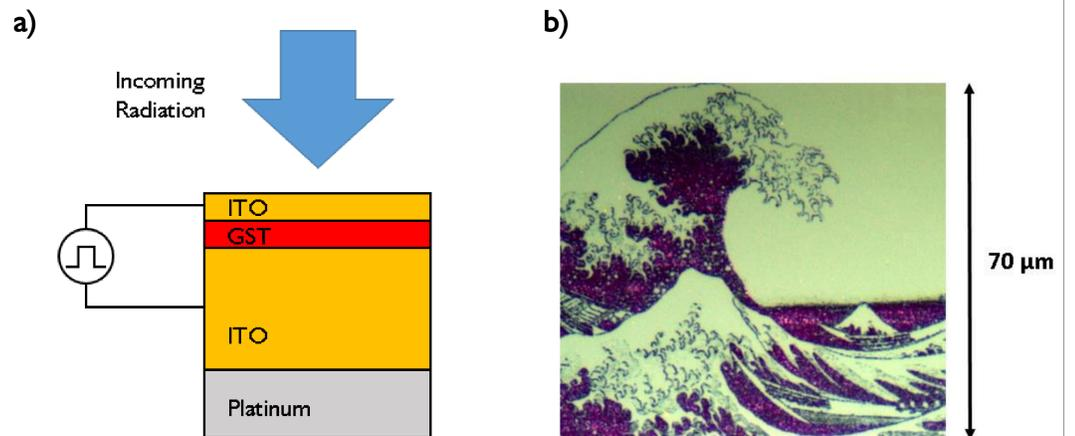
**Figure 1.** a) Phase-change display device structure proposed in [2], formed by a platinum bottom mirror and a GST layer sandwiched between two ITO layers. b) A high resolution ( $70 \times 70 \mu\text{m}$ ) image produced in such a structure produced changing the phase of the phase-change layer via Joule heating. The electrical pulse is sent employing an atomic force microscope in contact mode (CAFM).
