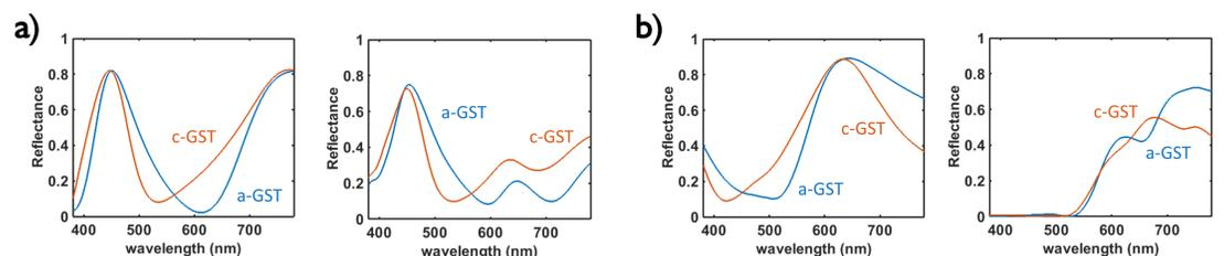
**Figure 3.** a) Reflectance spectra with the GST layer in amorphous and crystalline phases for the photonic cavity without (left) and with (right) the SRR. A reinforcement in blue wavelengths in the reflectance spectra caused by the interaction of the plasmonic resonator with the standing wave can be observed. b) Reflectance spectra of the photonic cavity without (left) and with (right) the array of strips; this structure attenuates blue wavelengths and preserve red wavelengths.
